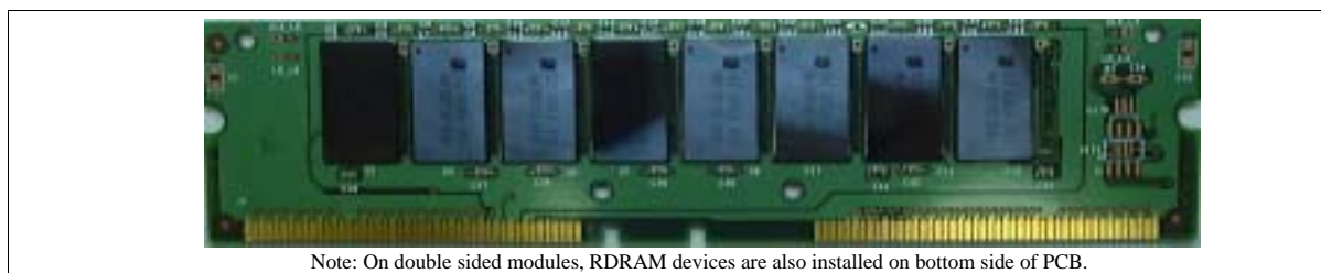
Figure 1: RIMM Module shown with heat spreader removed
